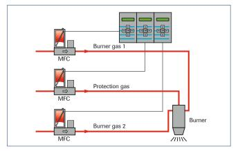
Burner control using Mass Flow Controllers brings many advantages compared to conventional systems, where flow is adjusted through needle valves. When burner orifices get clogged or when gas supply pressure varies, an MFC will automatically adapt to the changed conditions. For the control of relatively large flows with low differential pressure, which is typical for natural gas or  $CH_4$ , Bronkhorst High-Tech offers mass flow meters with separate pressure compensated bellows valves.
